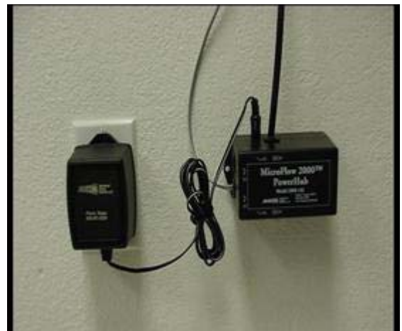
Figure 3. Transformer and PowerHub
